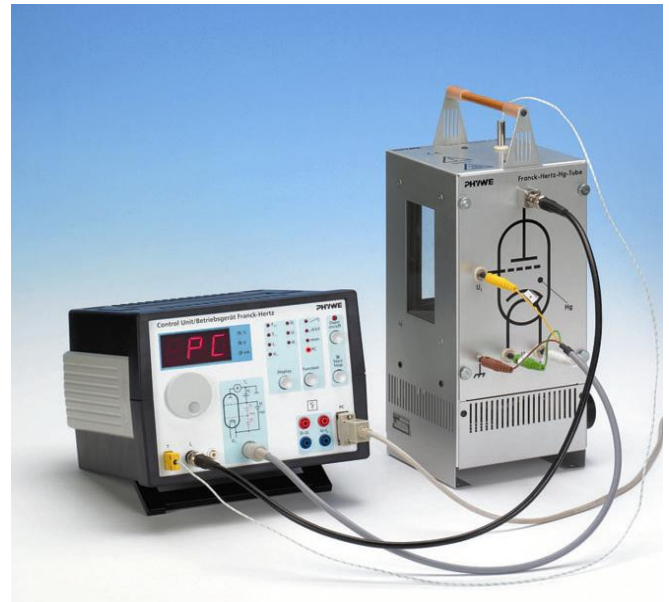
Fig. 2: Franck-Hertz experiment with Hg-Tube and oven
